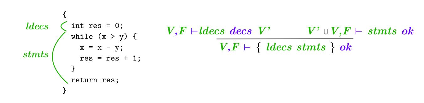
$\{x,y\},\{div:2\} \vdash ldecs \ ok \ \{x,y,res\},\{div:2\} \vdash stmts \ ok$
